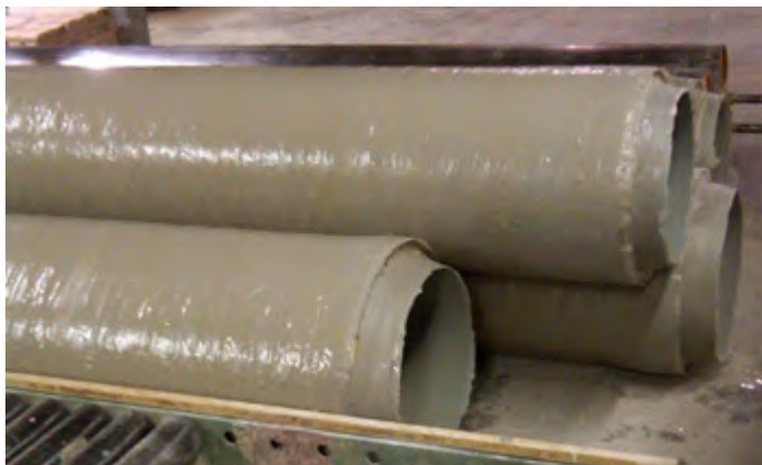
< UnderDuct, curing before heading to staging area
