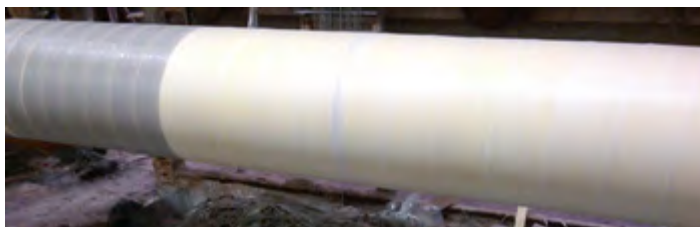
< UnderDuct, filament winding on mandrel
