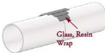
If additional lamination is to be made over a cured area, surface should be broken by sanding before application.
