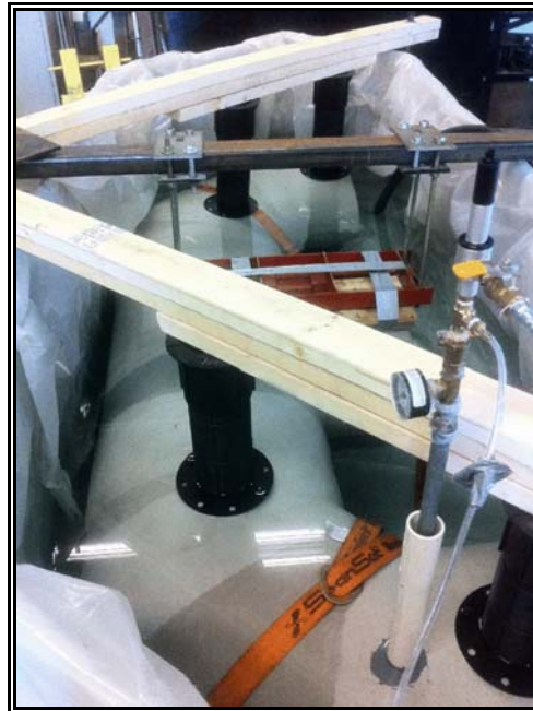
ICC-ES PMG LC1014, Leakage Test Fixture
