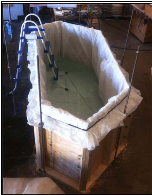
ICC-ES PMG LC1014, Leakage Test Fixture
